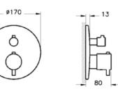
Minimax S built-in thermostatic 2-way mixer H: 170mm P: 80mm
