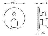
Minimax S built-in thermostatic 2-way mixer H: 170mm P: 80mm
